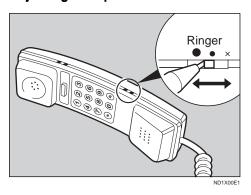
Adjust the optional handset ringer volume using the volume switch.
